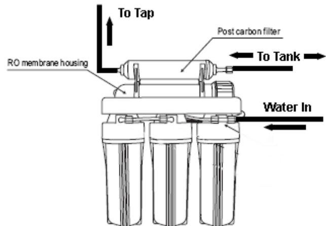
Hand tighten plastic shut-off valve to tank. Then connect tubing.
