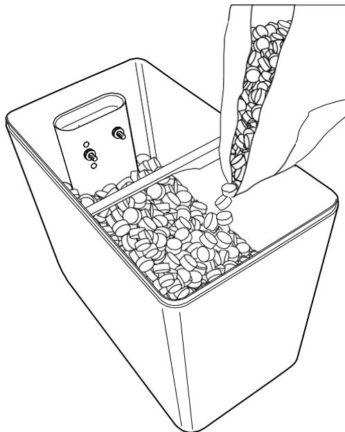
**DO NOT USE FINE OR GRANULAR SALT AS THIS WILL CAUSE A MALFUNCTION**
