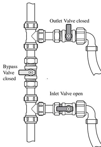
**Open the outlet valve. The inlet, outlet and bypass valves should now look like this.**
