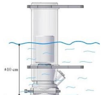
Slowly open the inlet valve to fill the resin cylinder. Open the nearest tap (that will be on softened water) and then slowly open the outlet valve. Alternatively turn the optional 'bypass' to 'service.'
