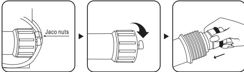
2. Turn off the water supply. Loosen the stainless steel pipe connector.
