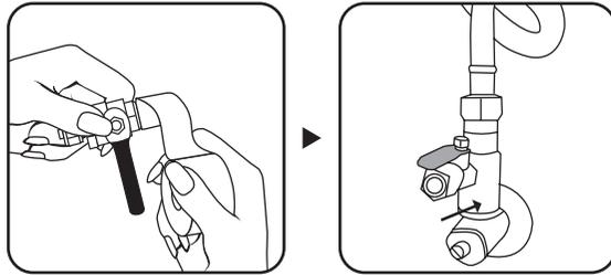
5. Get tubing white, connect it with deliver valve and the inlet water supply (as point 1 on page 07)
