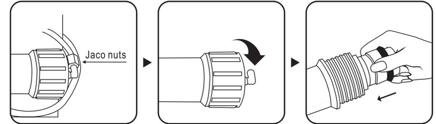
2. Turn off the water supply. Loosen the stainless steel pipe connector.
