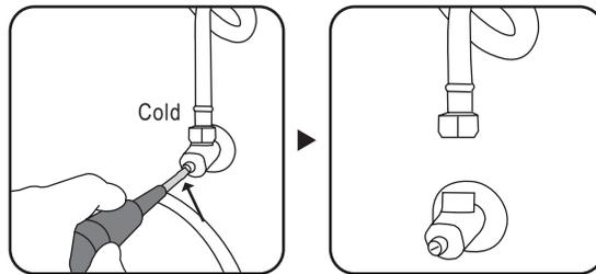
3. Get feed water connector and connect it to the stainless steel pipe as in the picture 2.
