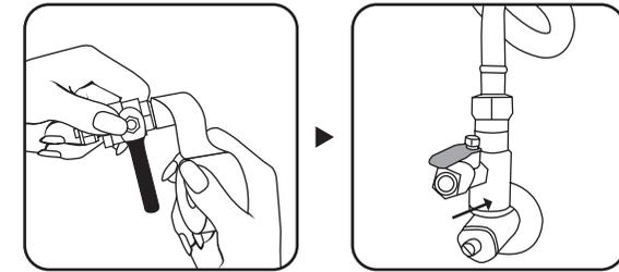
5. Get tubing white, connect it with deliver valve and the inlet water supply (as point 1 on page 06)
