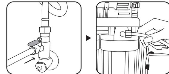
6.a. Unpack water storage tank. Take tank ball valve and deliver valve. Seal the female jaco fitting as attached on the water tank with Teflon tape for 15 circles. (picture 1). Take tank ball valve and tighten it up with the female jaco fitting.
