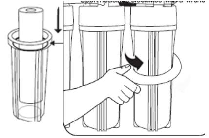
**Before fully tightening with the wrench, check that any o-rings are sited correctly.**
