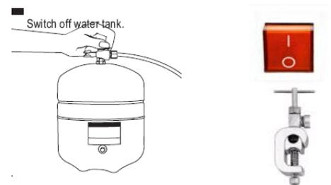
**You must open the tap connected to the system to relieve any pressure build up.**
