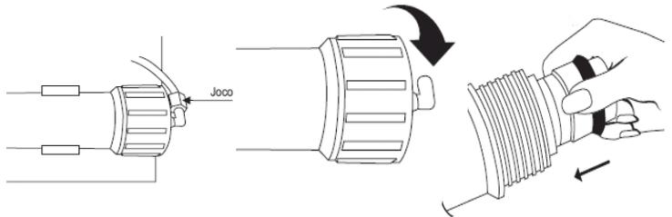
1. Remove the membrane housing cap.
